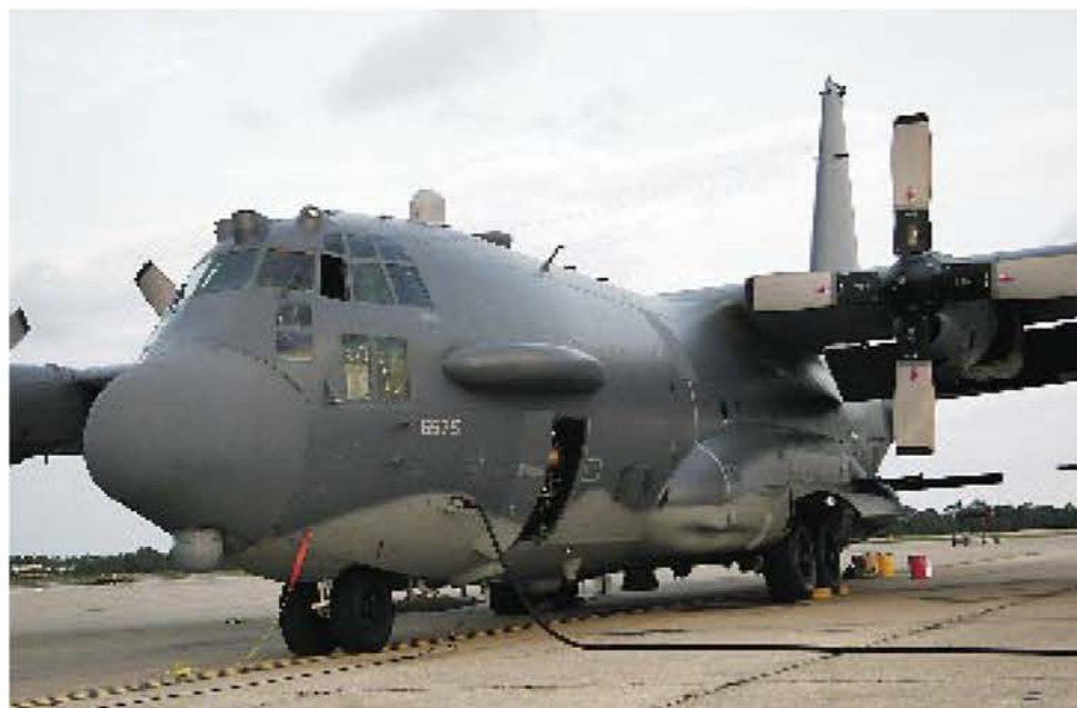
Top left, the AC-130's engines and external fuel tanks are clearly visible. Note the metal "bucket" covering the rear of the engine. These shrouds help block and suppress the heat signature of the aircraft's four turboprop engines. Top right are SSgt. Zachary Ross (l), A1C Aaron Lewis (in BDUs), and SSgt.
