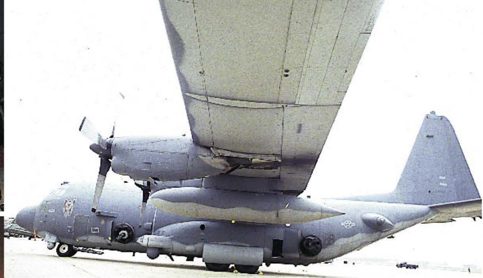
Above, the AC-130U weapons layout seen in profile. At the front is the 25 mm Gatling gun; the two larger caliber weapons are aft of the rear landing gear. AFSOC plans to soon replace the ancient 25 mm guns used on the AC-130Us with modern 30 mm Bushmasters offering better range, accuracy, and firepower.
